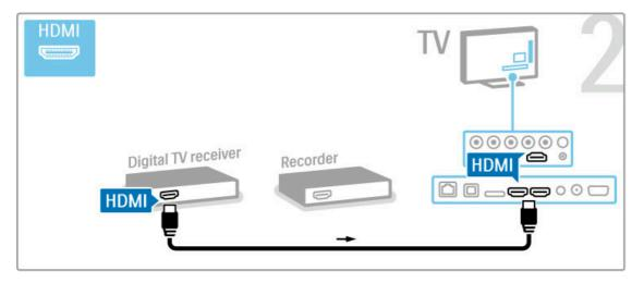
Finally, use an HDMI cable to connect the Disc Recorder to the  $\ensuremath{\mathsf{TV}}.$
